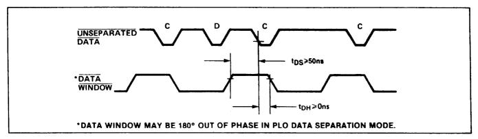
Figure 9. PLO Data Window Timing
