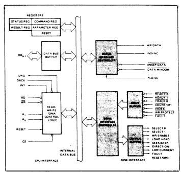
Figure 4. 8271 Block Diagram Showing Disk Interface Functions
