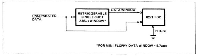
Figure 6. Single-Shot Data Separator Block Diagram
