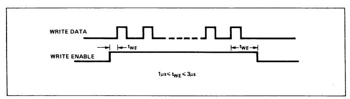
Figure 10. Write Enable Timing
