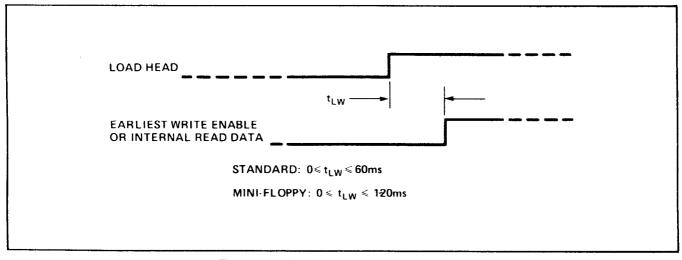
Figure 14. Head Load to Read/Write Timing
