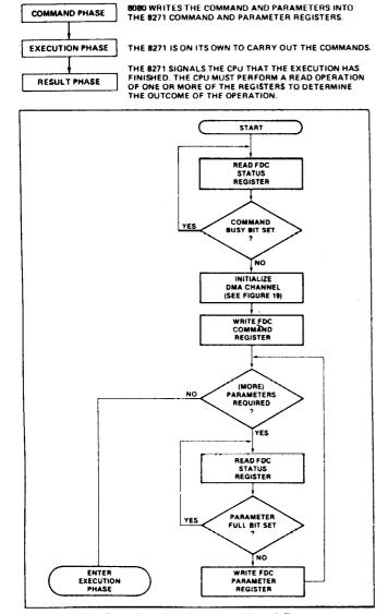
Figure 16. Passing the Command and Parameters to the 8271
