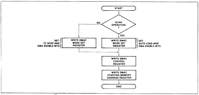
Figure 24. User DMA Channel Initialization Flowchart
