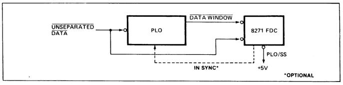
Figure 8. PLO Data Separator Block Diagram
