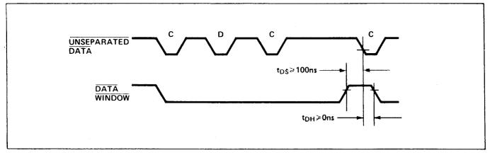
Figure 7. Single-Shot Data Window Timing
