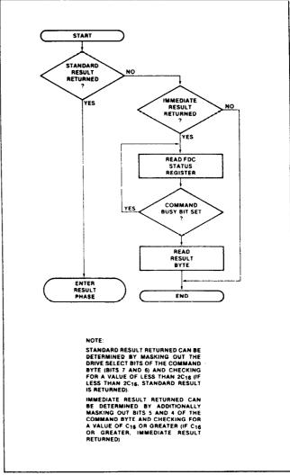
Figure 17. Checking for Result Type Following 8271
