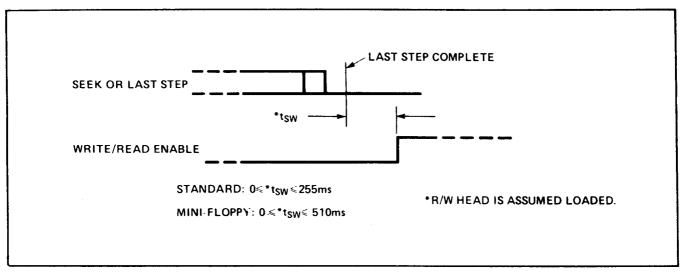
Figure 13. Head Load Settling Timing
