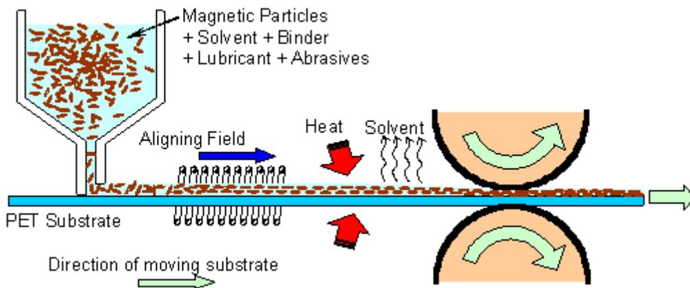
**Figure 14:** The processing route for particulate magnetic tape.
