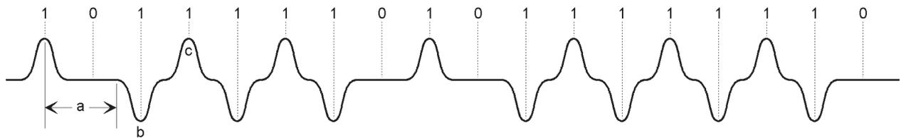
*When an interval is encountered during which no pulse occurs (see “a” above) the data separator “knows” that the next pulse must be a clock pulse (“b”). With the known clock pulse as a reference, the data pulses (“c”) can then be easily picked out and retained while the clock pulses are ignored.*
