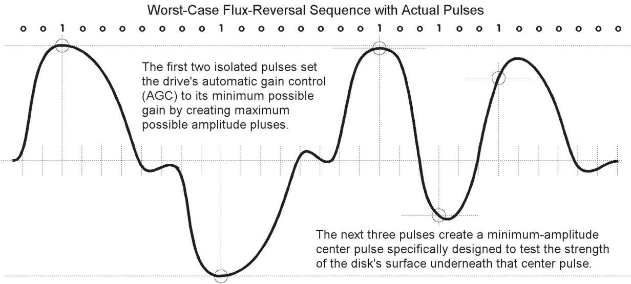
As you can see, the full-strength amplitude of the two isolated flux reversals is preserved, however the three closely-spaced pulses interact highly to produce a greatly reduced strength center pulse. This is the key to the first part of SpinRite's super-sensitive magnetic media surface analysis technology.
