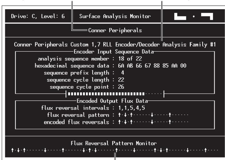
*The screen's "Encoded Output Flux Data" monitor shows the flux reversal patterns generated by the drive's flux encoder when presented with the Input Sequence Data.*
