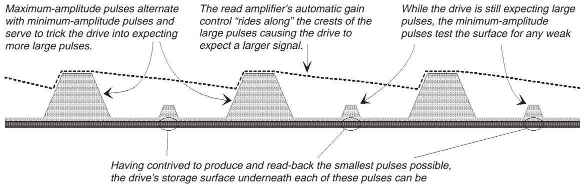
Since only the locations lying directly underneath the minimum-amplitude pulses are really being tested, a minimum-amplitude pulse must be successively placed over every possible flux-bit location of the drive. In other words, the special alternating large/small amplitude signal must be “slid along” the surface of the drive to search for all possible defects.
