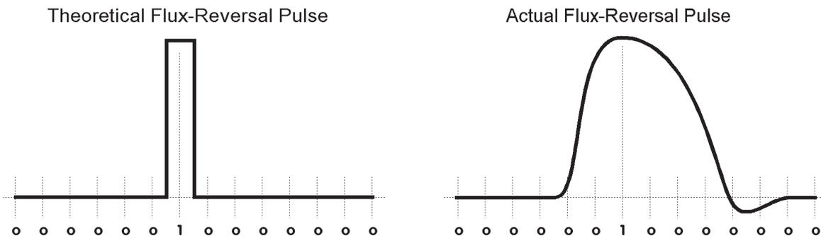
As you can see from the diagram above, whereas a theoretically perfect flux reversal pulse would be exactly one pulse-period wide, the pulse generated by an actual flux reversal has a much slower “attack” and “decay” time, and even dips a bit below the original signal level with behavior known as “overshoot.”
